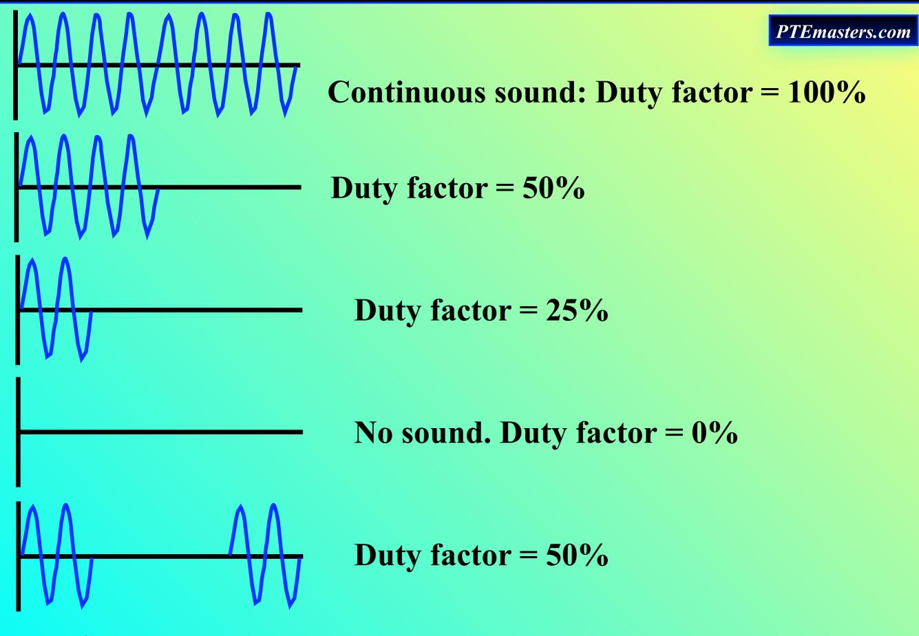
**Duty factor** is the fraction of time which an ultrasound system transmits a wave.
